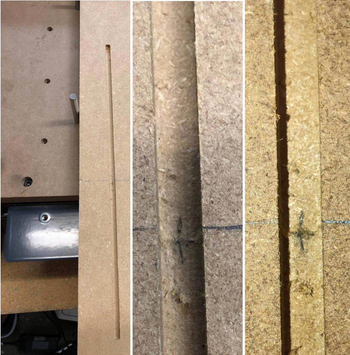
90 Deg V-Carve Bit, the horizontal lines are where the tiles intersect (Left line is a Rectangle on Easel and right line is a Line on Easel)
